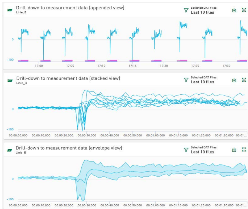
Several measurement files can be appended to each other (top) or compared directly in the stacked view (middle). In the envelope view (bottom), the maximum, mean and minimum values are displayed as trends.
