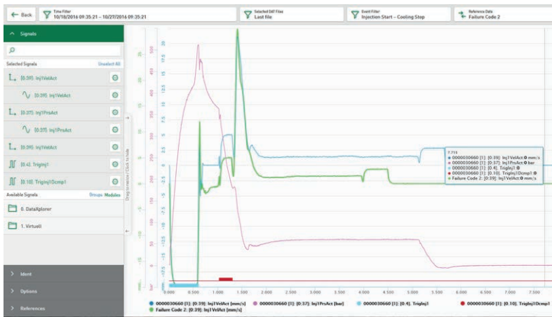
Current signal trends can be compared with reference signals (golden curve).
